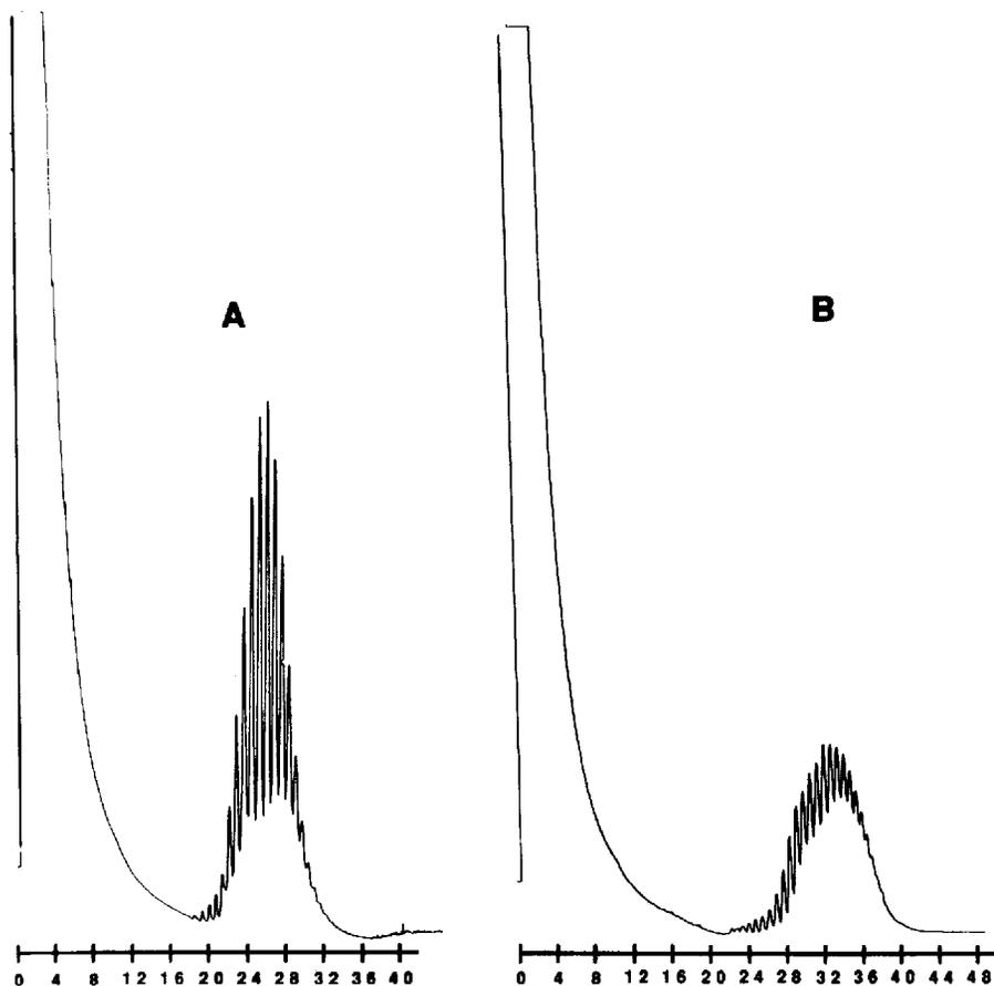
Fig. 6. Separation of standards of polyethylene glycol with an average molecular weight A = 600 and B = 1000 on a wide-pore octadecylsilanized packing (Vydac, 330 Å) coated with 3.5% (w/w) Ethoquad 18/25 and particle size 10  $\mu\text{m}$ . The column, 10 cm  $\times$  1 mm I.D. was packed by the displacement method. The mobile phase was carbon dioxide, temperature 80°C, and the pressure program 10 min at 100 atm increased linearly to 400 atm over 30 min.
