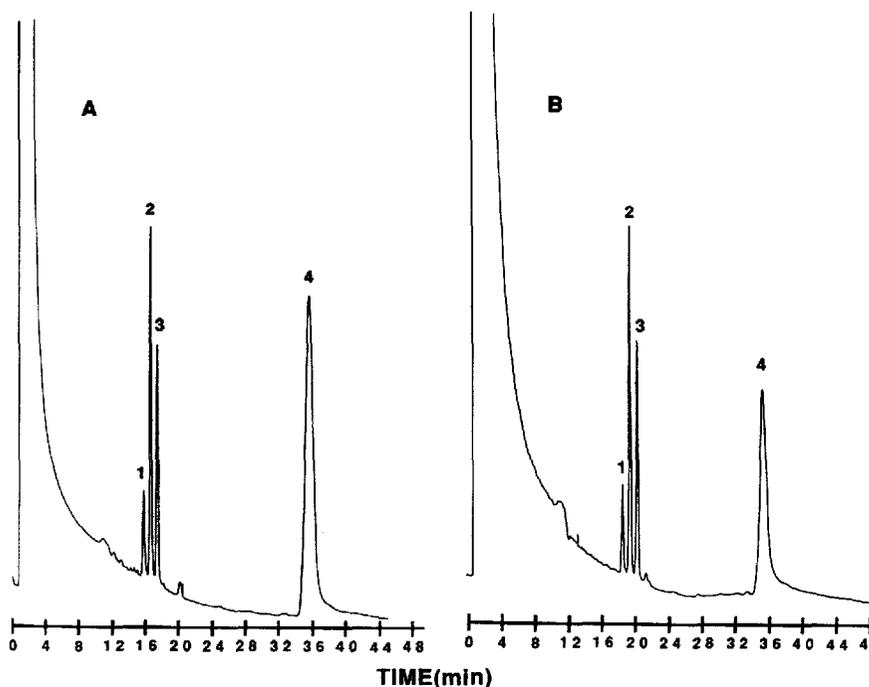
Fig. 9. Influence of silanol groups on the separation and recovery of 1 = cholestane; 2 = 5-cholestene; 3 = 3,5-cholestadiene, and 4 = cholesterol at A = 80°C and B = 100°C. The column was 10 cm  $\times$  1 mm I.D. packed with Corasil (II) by the tap-and-fill method. The mobile phase was carbon dioxide and the pressure program 10 min at 80 atm increased linearly to 300 atm over 30 min.
