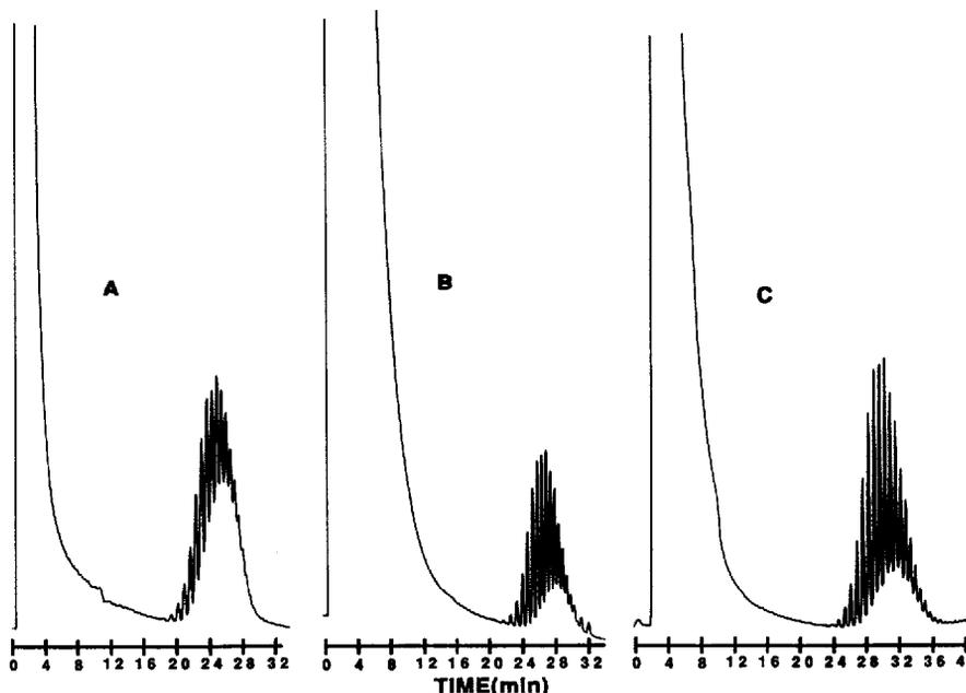
Fig. 2. The influence of column length on the resolution of a mixture of hydrocarbons extracted from parafilm with dichloromethane. The column lengths were A = 4 cm, B = 15 cm, and C = 30 cm, all of 1 mm I.D. Each column was packed with Alltech PC18 (37–55  $\mu$ m) by the tap-and-fill method. The samples were separated at 80°C, using carbon dioxide as the mobile phase and the following pressure program: 80 atm for 10 min and then linearly increased to 400 atm over 30 min.
