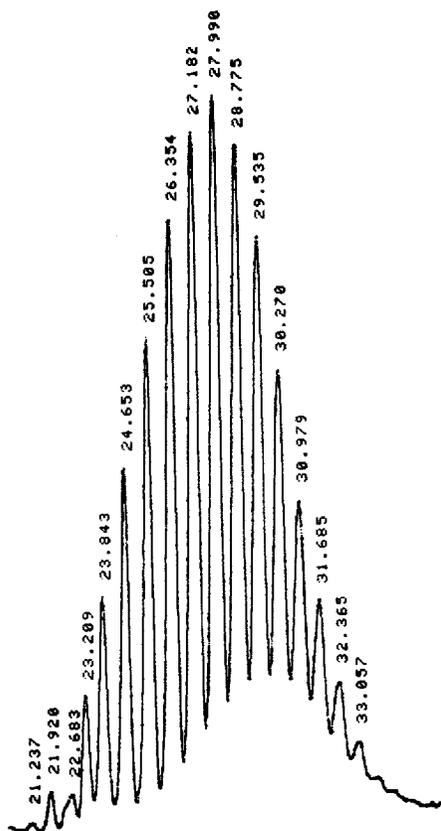
Fig. 11. Separation of Triton X-100 on a 10 cm  $\times$  1.0 mm I.D. column of Nucleosil 500, 10  $\mu$ m particle size, coated with a heavy loading of Ethoquad 18/25 (ca 20% w/w). The mobile phase was carbon dioxide, temperature, 80°C, and pressure program, 10 min at 80 atm, increased linearly to 450 atm over 30 min.
