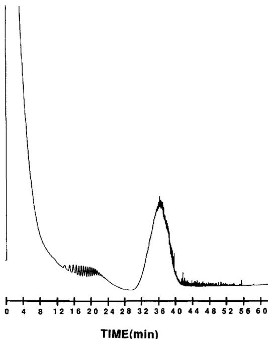
Fig. 7. Separation of a polypropylene glycol standard of average molecular weight 3010, contaminated with some oligomers of lower-molecular-weight material. The column was 7 cm  $\times$  1 mm I.D. The other conditions are identical with those for Fig. 6.
