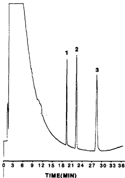
Fig. 12. Separation of 1 = cholestane, 2 = caffeine, and 3 = cholesterol on the same column and the same pressure program as that used for Fig. 11.
