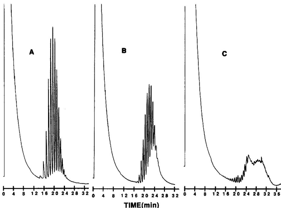
Fig. 5. The separation of polyethylene glycols of average molecular weight, A = 400, B = 600, and C = 1000. The column was 15 cm  $\times$  1 mm I.D. packed by tap-and-fill with Alltech PC18 + 0.4% (w/w) Ethoquad 18/25. The mobile phase was carbon dioxide; temperature 80°C, and the pressure program, 10 min at 100 atm, increased linearly to 400 atm over 30 min.
